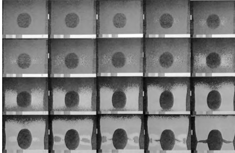
Figure 4.5: Deformation in a thin plate with a circular hole for twenty time instances during 20 seconds. Images 1-3 correspond to thermo-elastic cooling. Plastic heating begins at image 4 and continues up to image 16. Crack initiation and ductile fracture appear suddenly between images 16 and 17, (Bui, Ehrlacher and Nguyen, from an unpublished report 1979, Ecole Polytechnique)
